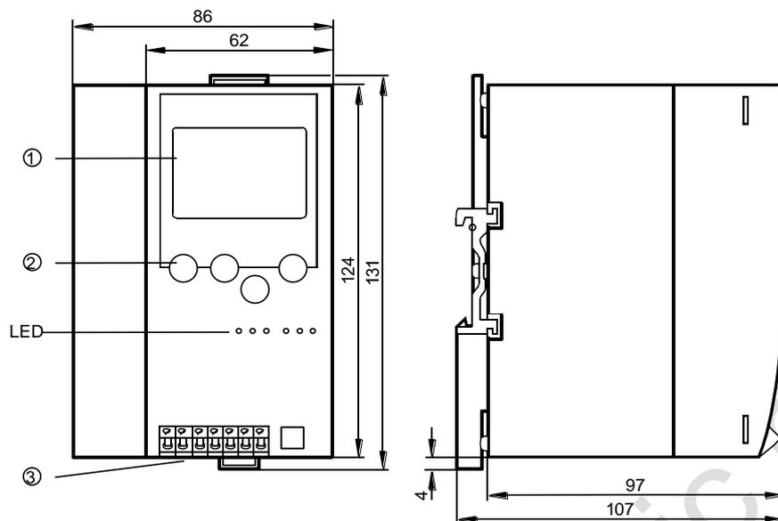
Figure: dimensions of the controller
