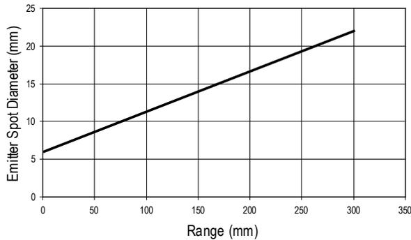
Figure 4. Typical Emitter Spot Diameter vs. Distance
