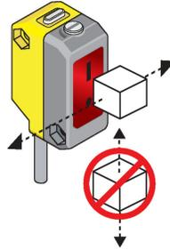
Figure 1. Optimal Orientation of Target to Sensor
