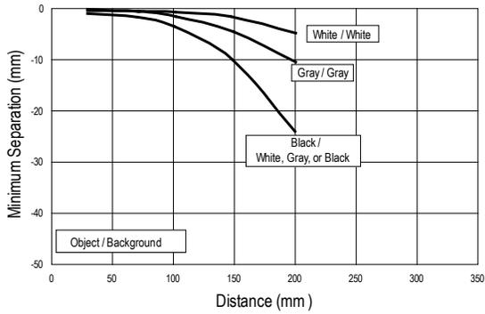
Figure 5. Minimum Separation Distance Between Object and Background
