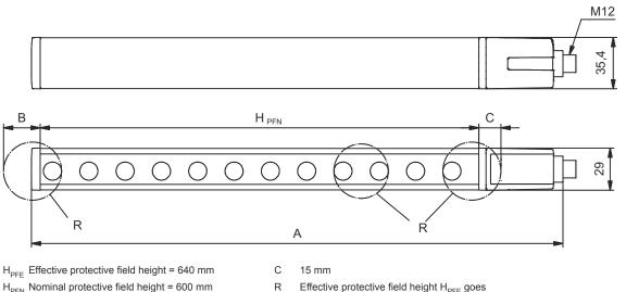
$H_{PFN}$  Nominal protective field height = 600 mm
