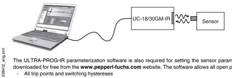
The ULTRA-PROG-IR parameterization software is also required for setting the sensor parameters. The ULTRA-PROG-IR software can be downloaded for free from the www.pepperl-fuchs.com website. The software allows all open parameters to be set, including:
