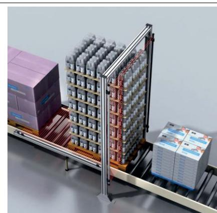
Figure 22: Detection of transparent objects
